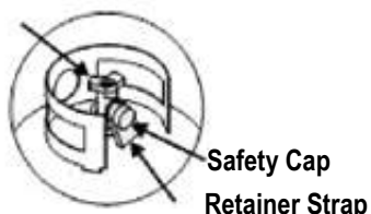
LP Tank Valve
